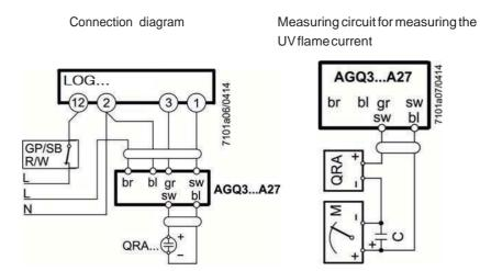
Measurement made at the flame detector QRA...
