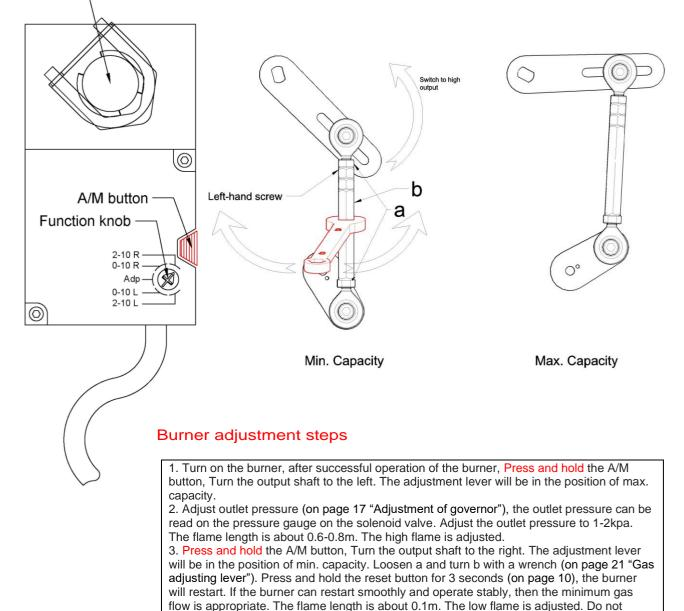
forget to tighten a again. 4. Release the A/M button and the flame of the burner will be automatically controlled by the actuator.
